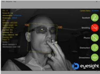
In April 2020, Eyesight upgraded its platform for incabin sensing solutions to detect when drivers who wear face masks get distracted or feel fatigued behind the wheel. It has developed a set of Al algorithms that can keep track of drivers' behavior behind the wheel when wearing masks, protection goggles or sunglasses. The company's Driver Sense and Fleet Sense leverage IR sensors to analyze head position, eye openness, pupil dilation, blink rate, and gaze direction, in any lighting condition.
