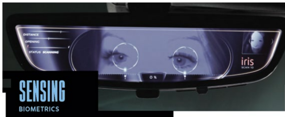
Gentex Full Display Mirror with Iris Recognition Technology
