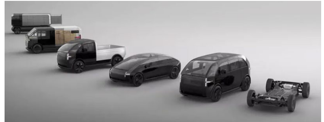
KIA bodystyles enabled by Canoo's modular skateboard platform
