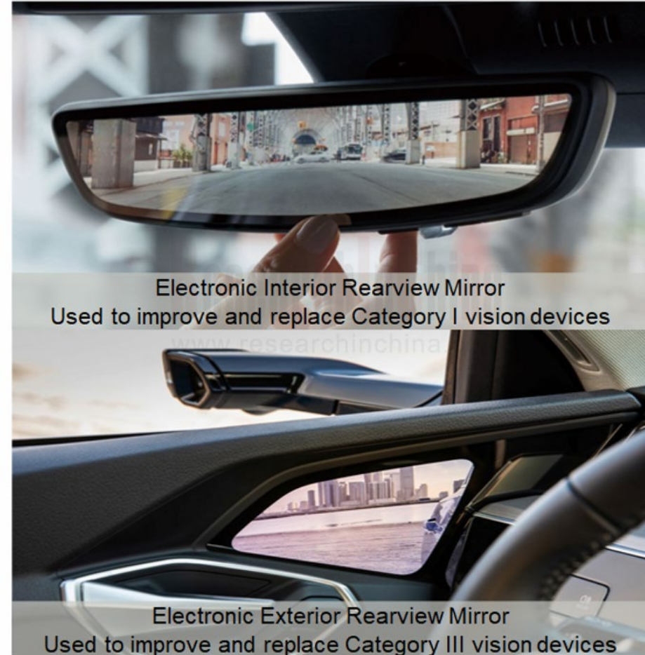
Electronic Rearview Mirror Diagram (Take a Passenger Car as an Example)
