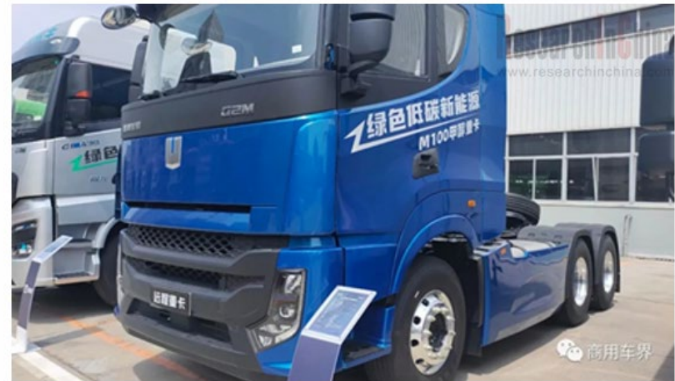
Geely remote G2M methanol tractor, over 1000km range
