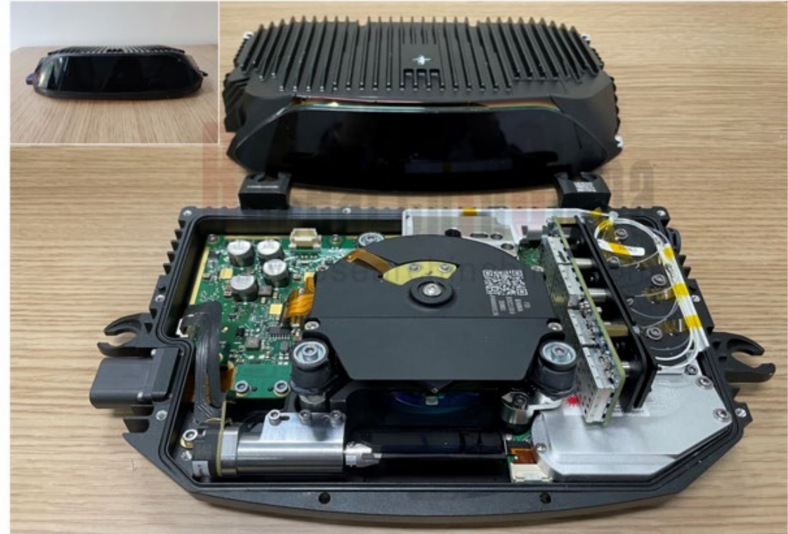
Internal structure of the Innovusion Falcon LIDAR installed in the NIO ET7 model
